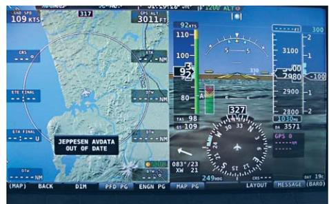
Pilot interface with the PFD and EMS is by way of two joystick controls and eight contextual buttons on the bottom of the bezel (the button menus change depending on the options chosen by the pilot). The joysticks are easy to use, for instance in selecting waypoints on the moving map to construct your
