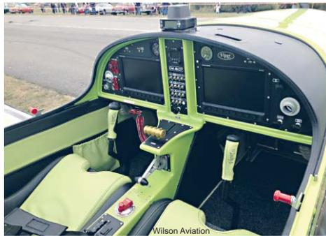
The cockpit layout is typical microlight/LSA, with red ballistic recovery chute handle in immediately front of the pilot. The portable collision avoidance system (PCAS) is useful for locating a camera aircraft which has set out from a separate airfield.
